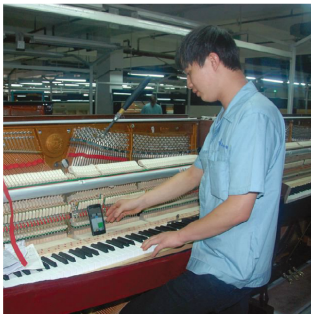
Left, workers at Hailun's new factory set and regulate the actions on uprights in production. Right, a sign of the times: a piano is tuned by smartphone app.
