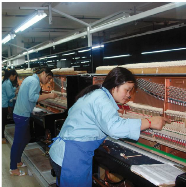
Left, workers at Hailun's new factory set and regulate the actions on uprights in production. Right, a sign of the times: a piano is tuned by smartphone app.
