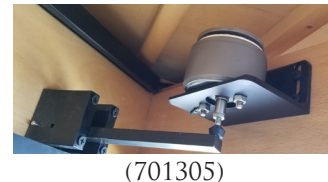
PNOMation Sustain Pedal Solenoid
